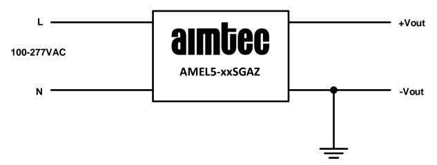
AMEL5-xxSGAZ models meet the EN55022 class B compliance when connected to Earth/Ground. These models are incorporating an EMC compliant filter and when connected to Earth/GND, no external filtering will be needed to meet the specified limits.
