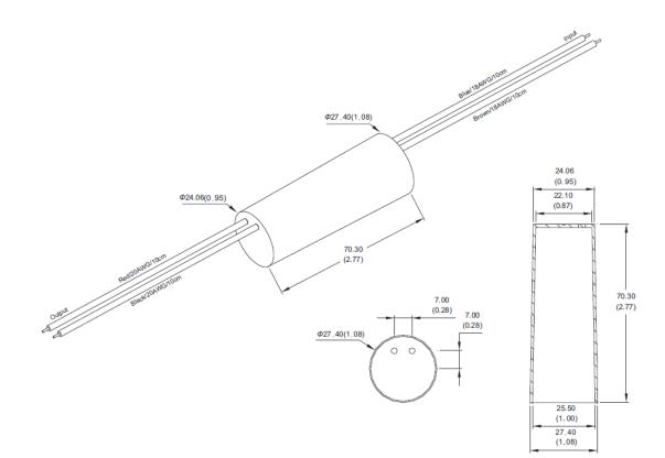
Dimensions mm (inch) Case Tolerance ±0.50 (±0.02)
