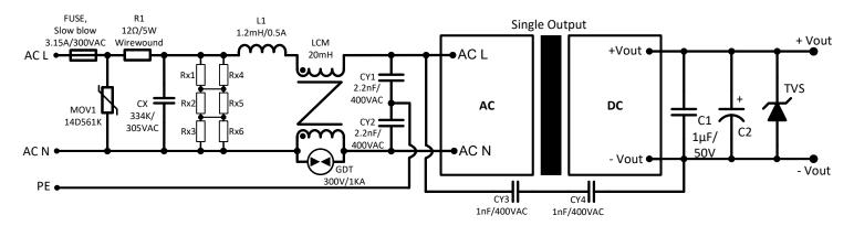
Rx1, Rx2, Rx3, Rx4, Rx5, Rx6 1.5MΩ/150VDC/1206
