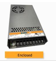
The AMES350-NZ is Aimtec's highest power AC/DC converter that offers much greater cost effectiveness due to material normalization and production automation also leading to improved reliability and performance. Offering a commercial input voltage range of 90-264VAC and an output voltage range from 5-48V, this series will offer many benefits to your new system design.
