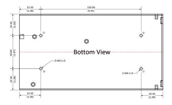
Note: Unit: mm(inch) Wire gauge: 22-12AWG Screw terminal tightening torque: M3.5, 0.8N-m Mounting screw tightening torque: M4, 0.9N-m General tolerance:  $\pm 1.0(\pm 0.04)$ At least one of the (1) - (8) location must be connected to PE
