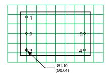
Dimensions mm (inch). Pin diameter tolerance  $\pm 0.1$  ( $\pm 0.004$ ) Pin height tolerance  $\pm 0.5$  ( $\pm 0.02$ )
