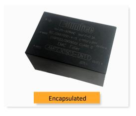
Aimtec's AMFE30503 series is designed to offer protection against AC power surges. These filters can assist the AC-DC converters in meeting the Surge level of IEC/EN61000-4-5 standard ±1KV (2Ω internal resistance) or ±2KV (12Ω internal resistance) and EMI requirement of CISPR22/EN55022 Class B standard.
