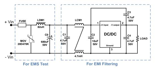
The part choice of the FUSE is based on actual input current.
