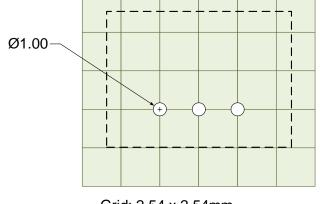
Grid: 2.54 x 2.54mm Unit:mm[inch] General tolerances:±0.5mm [± 0.020inch]
