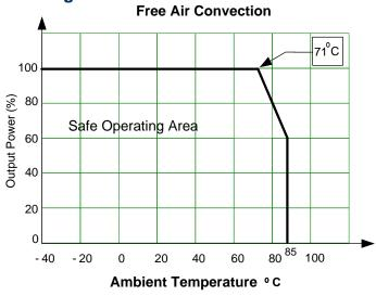
NOTE: With air convection speed of 0.8m/sec
