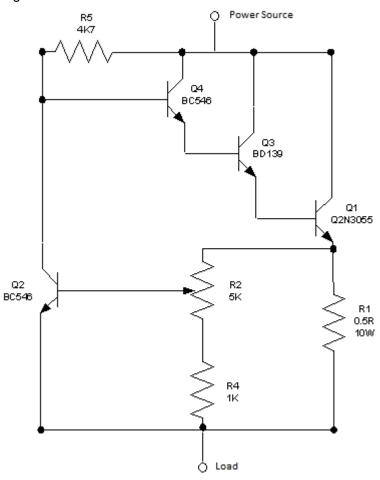
R1 is the current sense resistor. When R2 potentiometer is at minimum resistance (the center tap connected to R1), and the current drawn by the load reaches 1.2A the voltage across R1 will reach 0.6V and Q2 begins to conduct current and shorts the base voltage of Q4 to ground. The shorting of Q4 base to ground reduces the base current and the output voltage sensed by the load, preventing the current from flowing further.
